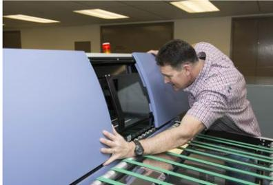
A laser will flash text on the chemical coated aluminum plate in the chamber - burning the chemical on the plate.
