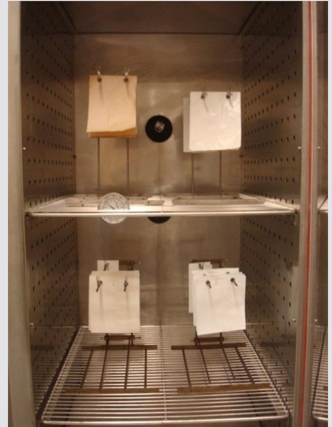
Aging of coated and uncoated papers in a temperature and humidity controlled oven.
