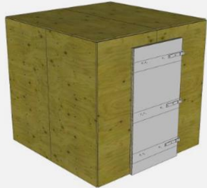
Figure 3. Safe room with plywood nailed and glued to lumber beams.
